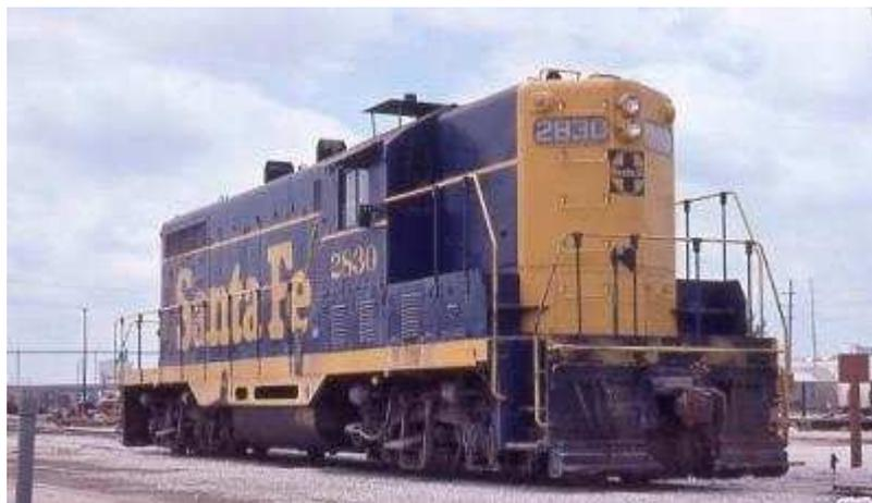
In 1980 the 2830 was rebuilt with a low hood, repainted in the traditional Santa Fe "War Bonnet" and renumbered, **ATSF 1312**. At this point the ATSF 1312 was used for yard service in this "Cow-Calf" configuration. (1312 on the left)
